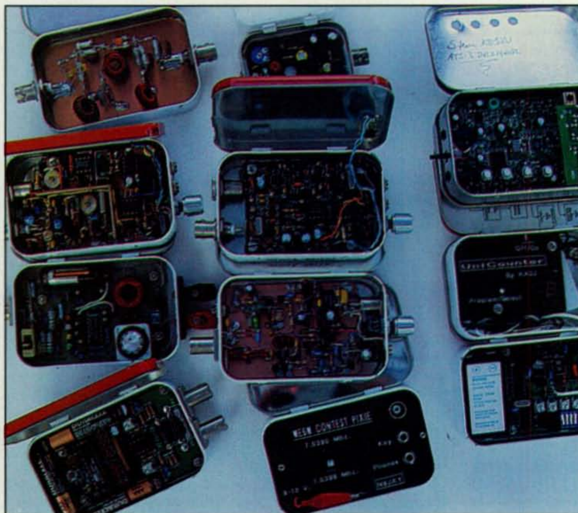
Photo G— Some of the neat mini rigs Dennis Payton, N9JXY, built and installed in Altoids® tins. Included in this view are: the famous W7ZOI Micro Mountaineer transceiver (second from top on left), a WE6W Pixie transceiver (bottom center), an 80-meter transceiver, a 40-meter Rockmite above it, and a digitally tuned transceiver (upper right). (Photo courtesy of N9JXY)
