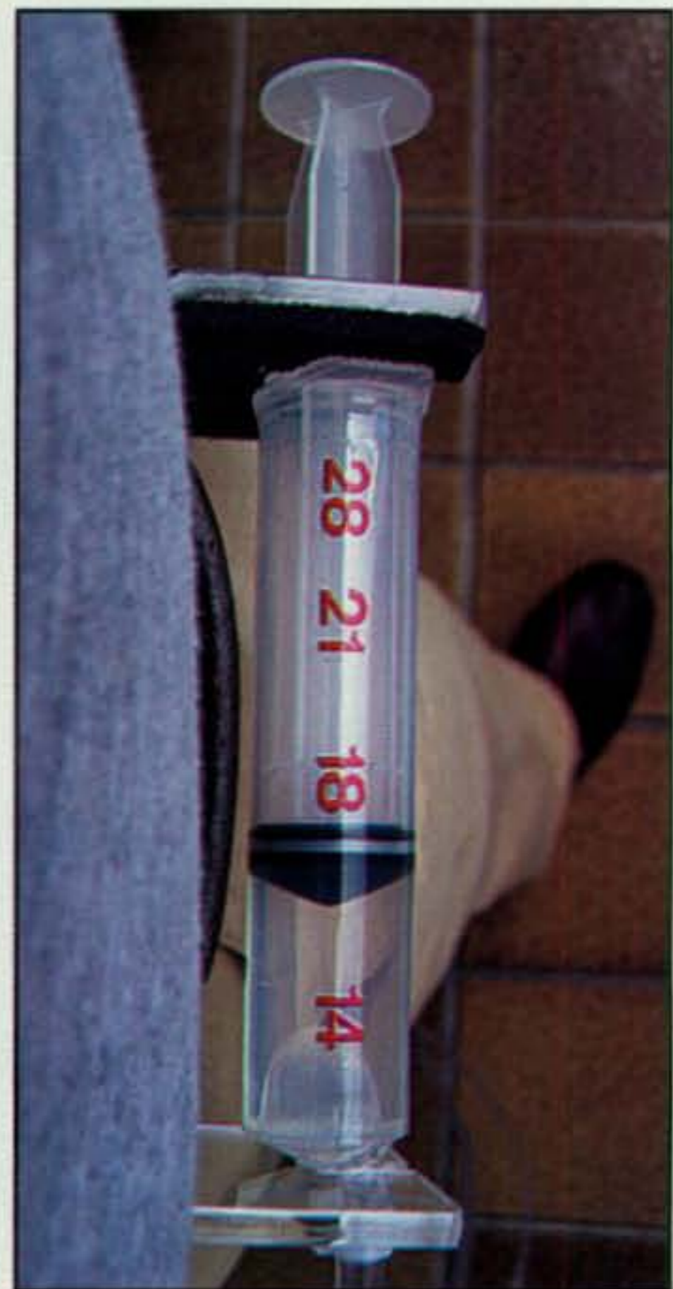
Photo E— A second syringe marked in megahertz is fitted with a belt clip and connected to the loop-mounted syringe via a plastic tube filled with water. This is the view looking down from Alex's shoulder. (Photo courtesy of PY1AHD)
