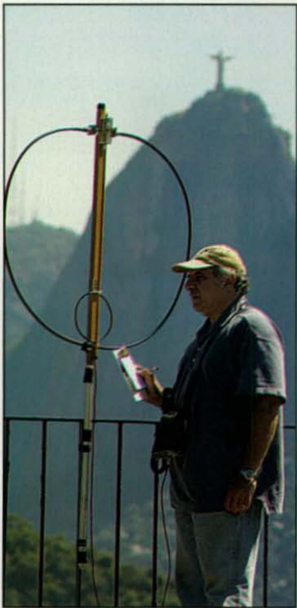
Photo C— Alex Grimberg, PY1AHD, has made over 500 DX contacts while operating personal portable with a Yaesu FT-817 and his water-tuned loop antenna shown here and described in the text. Notice the background, friends: That is a 38-meter tall statue of Christ overlooking Rio de Janeiro from atop Corcovado Mountain, which is the tallest point in the area. It is a world-famous landmark comparable to the Statue of Liberty in New York City, the Eiffel Tower, etc. (Photo courtesy of PY1AHD)
